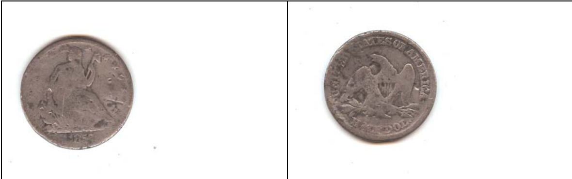
Figure 1 – Counterfeit 1857 Half Dollar. Measured diameter: 30.5 mm (correct 30.61 mm). Measured weight 8.75 gm ( correct 12.441 gm).
